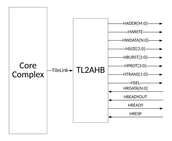
Figure 1: TL2AHB Block Diagram
