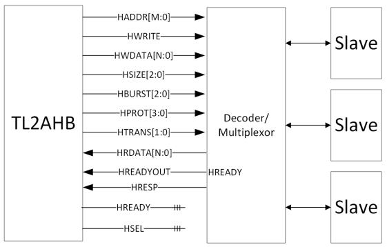
Figure 3: TL2AHB connected directly to a slave
