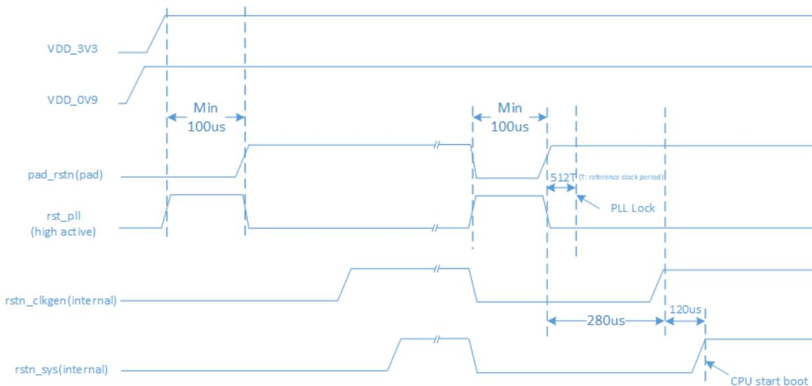
Figure 8-1 Reset timing
