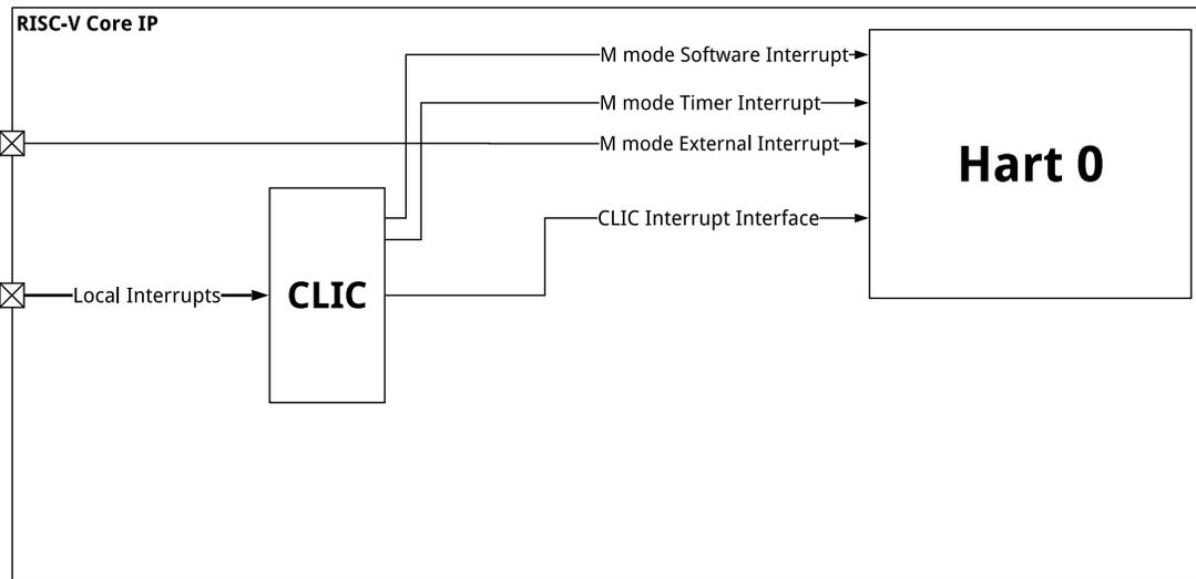
Figure 2: VIC\_E24 Interrupt Architecture Block Diagram.
