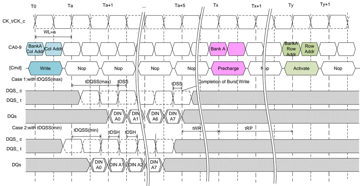
Figure 13-6 LPDDR3 Burst Write
