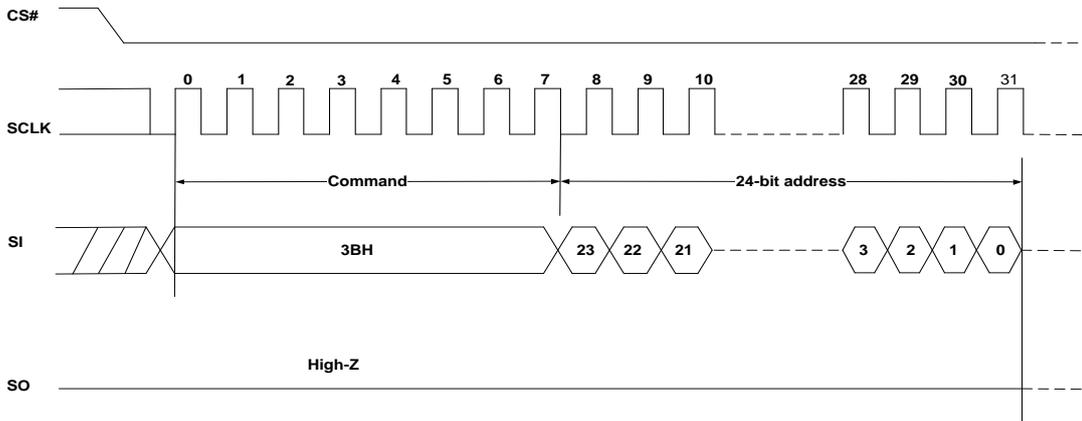
**Figure 13-14 SPI Write**
