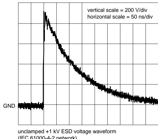
unclamped +1 kV ESD voltage waveform
