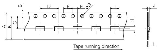
Taping condition : Lack of products in the middle of taping should be one MAX, but total quantity specified in the specifications should be secured.
