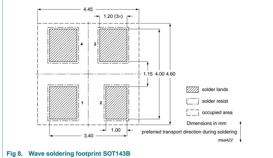
Fig 8. Wave soldering footprint SOT143B
