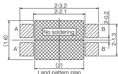
Soldering thickness  $t=0.08\pm0.01$
