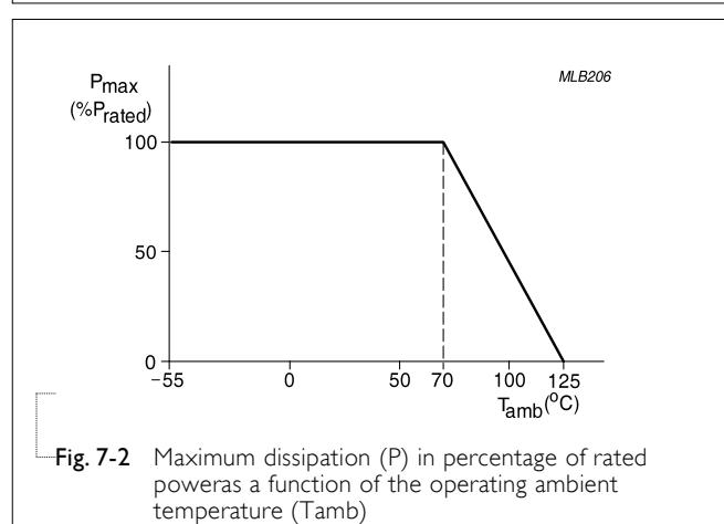
Fig. 7-2 Maximum dissipation (P) in percentage of rated power as a function of the operating ambient temperature (T<sub>amb</sub>)
