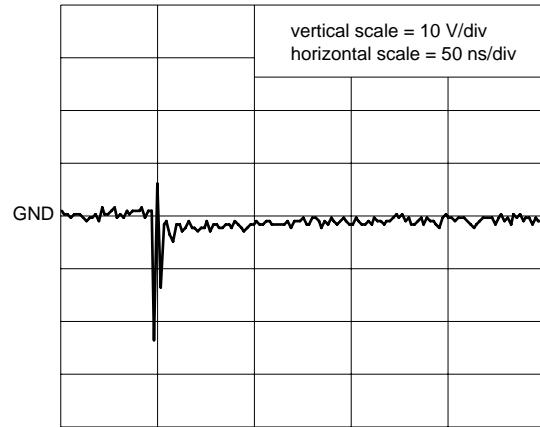
clamped -1 kV ESD voltage waveform
