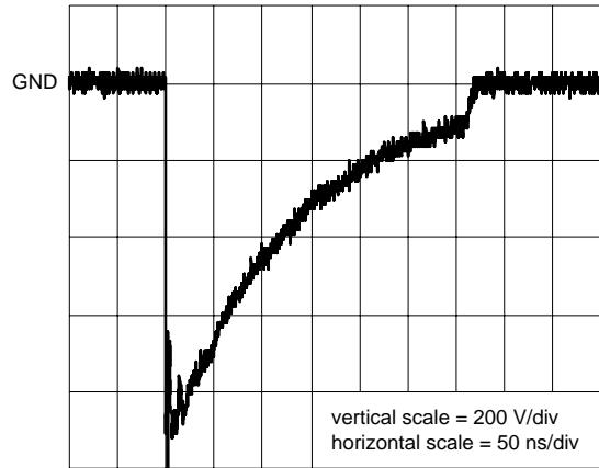
unclamped -1 kV ESD voltage waveform
