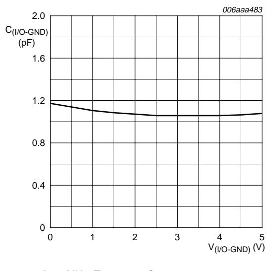
$f = 1\text{ MHz}; T_{amb} = 25^\circ C$
