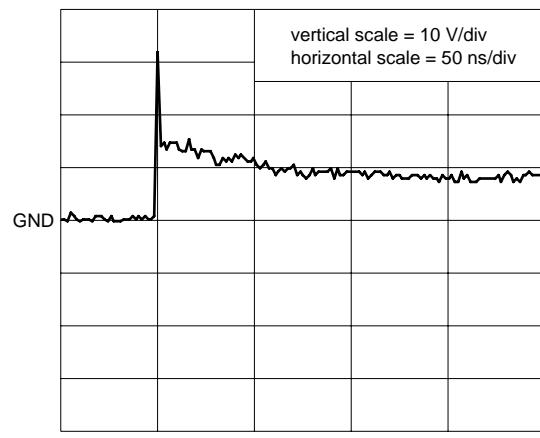
clamped +1 kV ESD voltage waveform
