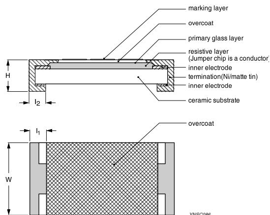
Fig. 6 Chip resistor outlines
