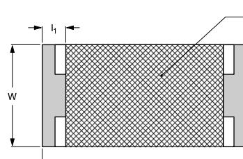
Fig. 6 Chip resistor outlines
