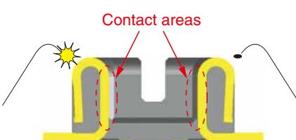
Contact areas are not exposed to the outside penetration of the flux or other physical particles.
