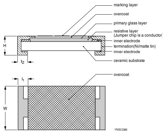
Fig. 6 Chip resistor outlines
