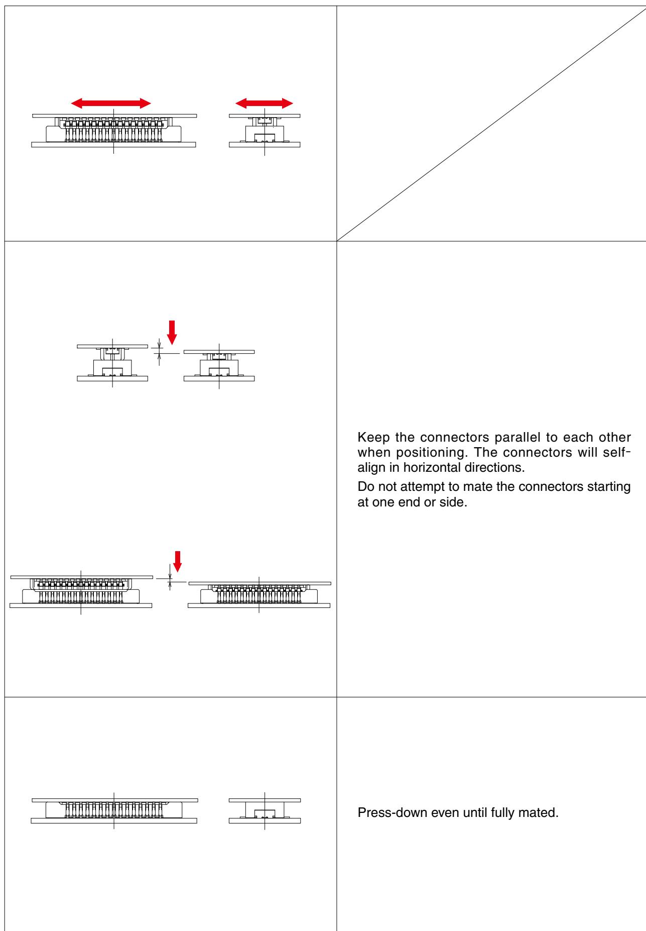
Keep the connectors parallel to each other when positioning. The connectors will self-align in horizontal directions.
