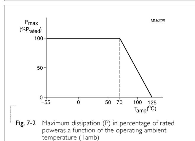
Fig. 7-2 Maximum dissipation (P) in percentage of rated power as a function of the operating ambient temperature (T<sub>amb</sub>)
