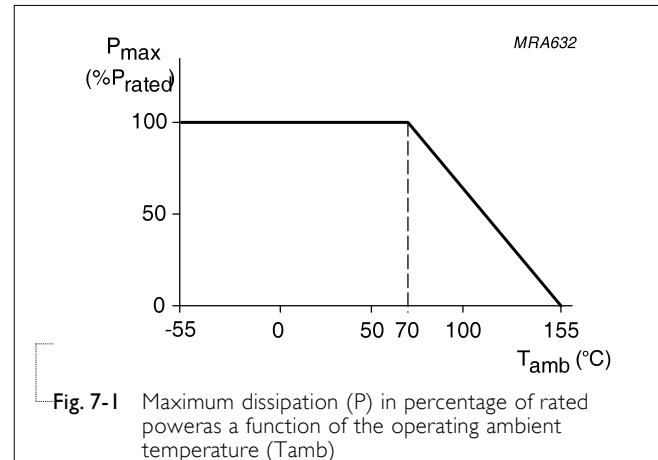
Fig. 7-1 Maximum dissipation (P) in percentage of rated power as a function of the operating ambient temperature (T<sub>amb</sub>)
