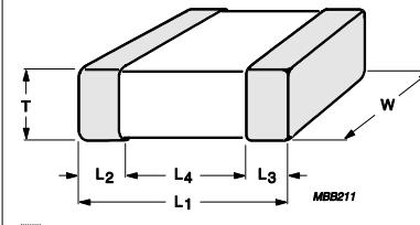
Fig. 2 Surface mounted multilayer ceramic c
