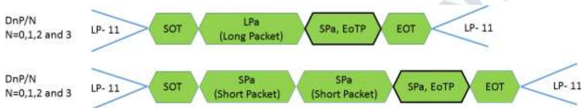
Figure 5-54 End of Transmission Packet (EoTP) – Example
